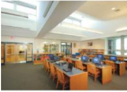
Twenhohel is the first school in Kentucky oriented to take maximum advantage of daylighting. Windows supplement artificial lighting in the media center and throughout the school. Before Twenhohel's construction, most Kentucky schools were oriented with the street.
