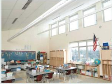
The Kenton County School District constructed Caywood Elementary at the same time that it built Twenhofel. Caywood was designed differently, with all daylighting glazing integrated in the exterior wall and oriented to the south.
